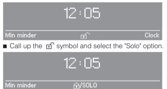
The  $\ensuremath{\underline{n}}$  /SOLO symbol indicates that the solo programme has been activated.
